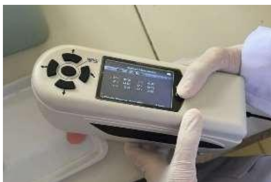
Figure 2. Measurement of thermoplastic nylon color using a colorimeter
